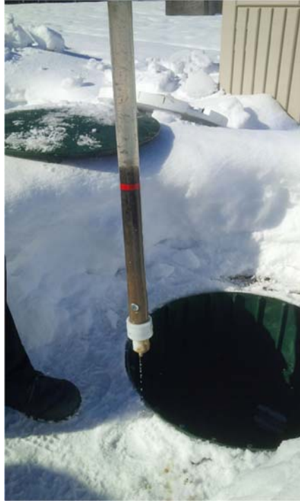
Figure 5b. The digester still has insufficient solids to warrant a pump out, after 18 months of continuous peak flow.
