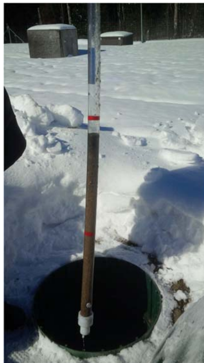
Figure 5a. In 10 months after its first pump-out, the septic tank is completely full of solids.
