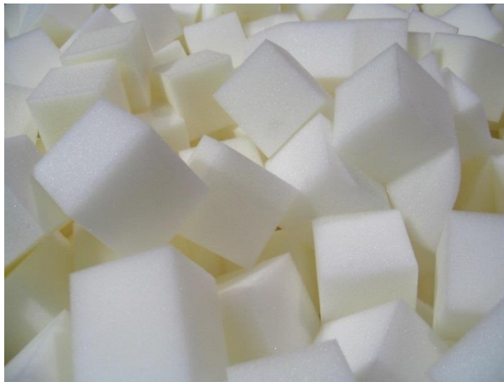
Figure 1. Waterloo Biofilter foam filter media
