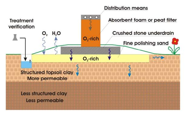
Absorbent attached-growth biological filters, such as open-cell foam or sphagnum peat, operate similar to natural soils but use a manufactured filter medium with properties
