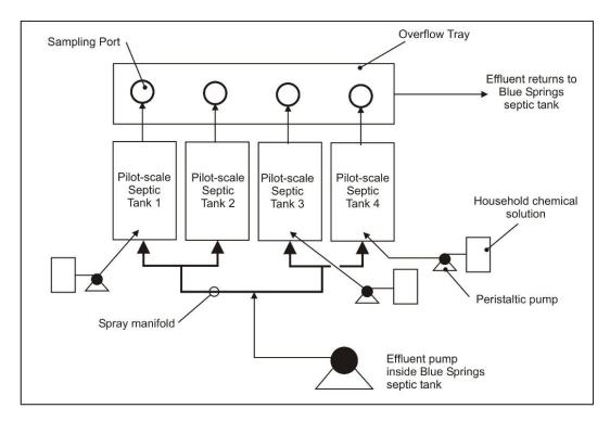
Figure 2. Layout Schematic of the Experimental Apparatus
