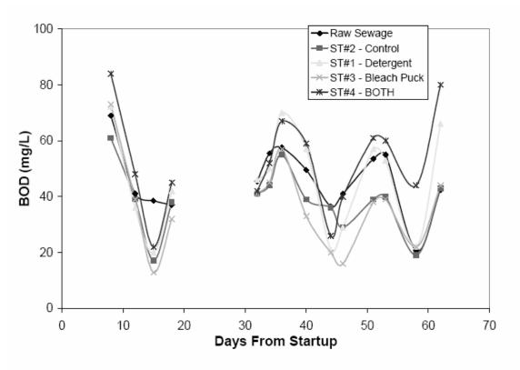
Figure 3b. Set B (Chemicals Dosed) – Raw Sewage and Effluent BOD
