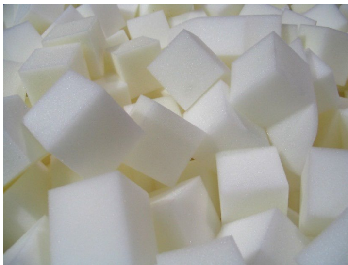
Figure 1. Waterloo Biofilter foam filter media
