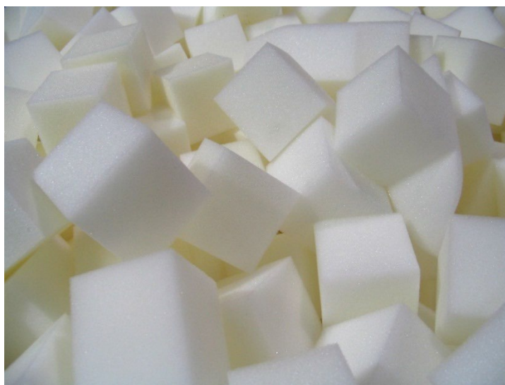
Figure 1. Waterloo Biofilter foam filter media
